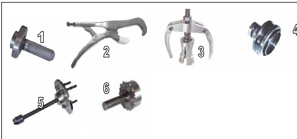
1. tool for roller bearing to fit in.
